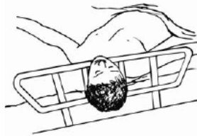
Zone 3 – Entrapment between the rail and the mattress
