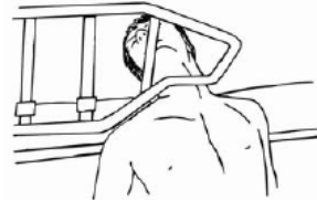
Zone 6 – Entrapment between the end of the rail and the side edge of the head or foot board
