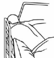
Zone 6 – Entrapment between the end of the rail and the side edge of the head or foot board
